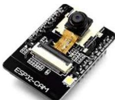
Gambar 2. Esp32Cam
