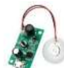
Gambar 1. Ultrasonik Mist Maker [7]
