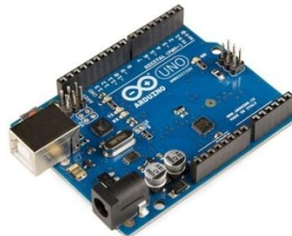
Gambar 4. Board Arduino Uno
