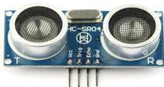
Gambar 6 Sensor HC-SR04 Ultrasonic
