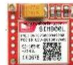
Gambar 3. Modul GSM 800L v1 [13]
