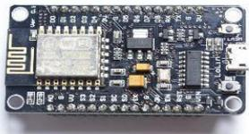
Gambar 2 NodeMCU ESP8266
