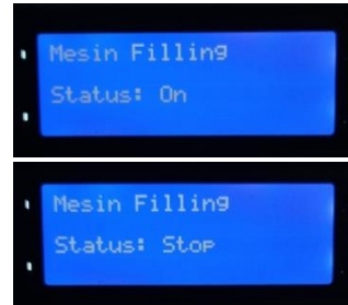
Gambar 7. Implementasi program Water Pump
