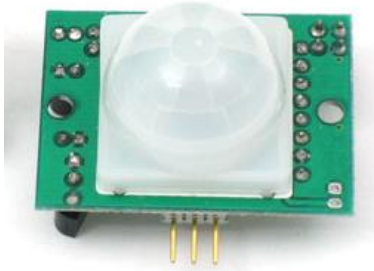
Figure 3 Passive Infrared Sensor (PIR) [14]
