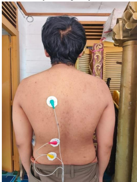
Figure 4. The placement of the electrode pad from EMG sensor to measure the back muscle signal
